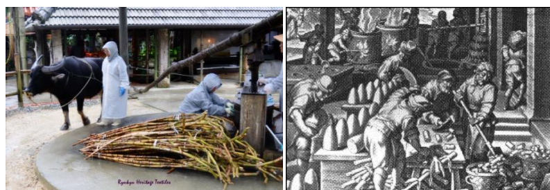
Ancient ways to extract sugar from cane, still used today by artisans (left); and (right) a European mediaeval factory for the manufacture of sugar, with 'loaves' seen lined up at left to be sent for sale
